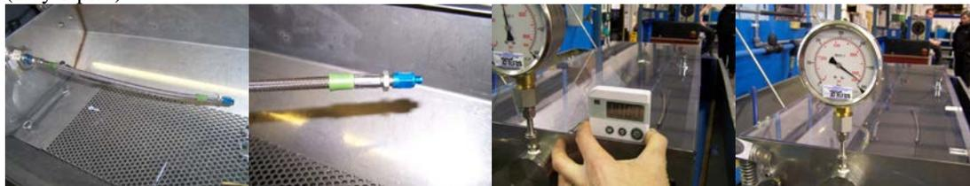
Assy 2 – 4000psi held for 2 mins – no failures observed
